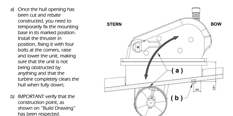
c) Once completely satisfied with the position and height of the mounting base, the base can be permanently stratified and fixed into the hull while respecting the inside dimensions of the mounting base. In order to ensure that the mounting base keeps its initial form during the stratification process, one can use some wooden spacers (length = 249 mm) on the inside of the mounting base.
