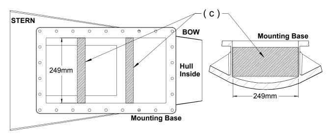
d) The reason for respecting these dimensions is to avoid the sliding plates becoming Thruster wedged into mounting base Unit resulting in the unit getting stuck in the down position. e) Before fixing the thruster unit onto the mounting base flange it is important to Sliding ensure that the top surface Plates of the mounting base flange is perfectly flat to accept the « O » ring seal of the (d) d ) Compact Retract base flange ensuring perfect water tightness. 249mm at top 249mm at bottom
