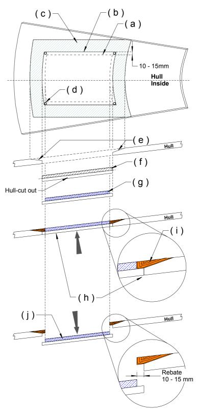
j) Once rebate is set, remove the male plug. Now remove temporarily fixed piece of wood from shaved down hull cut-out and keep the hull cut-out to use as closing plate.
