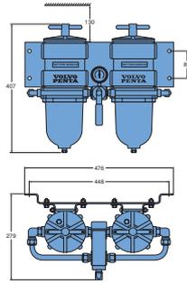
**Double fuel filter/water separator, diesel engines**
