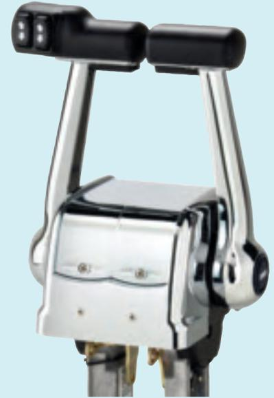
**Top-mounted controls for twin installation**
