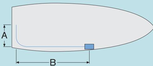
It is very important to select the exact cable length, fewer bends mean better operation and durability. Measure, in as straight a line as possible, the distance between the control mechanism and the engine/transmission connections. Calculate a radius of 200 mm for all bends. Adapt the cable as shown in the illustration  $L = A + B + 200$  mm. If the measurement falls between two standard cable lengths, select the longer cable.
