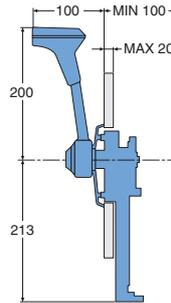
**Control lever assembly PC-841, side-mounted**
